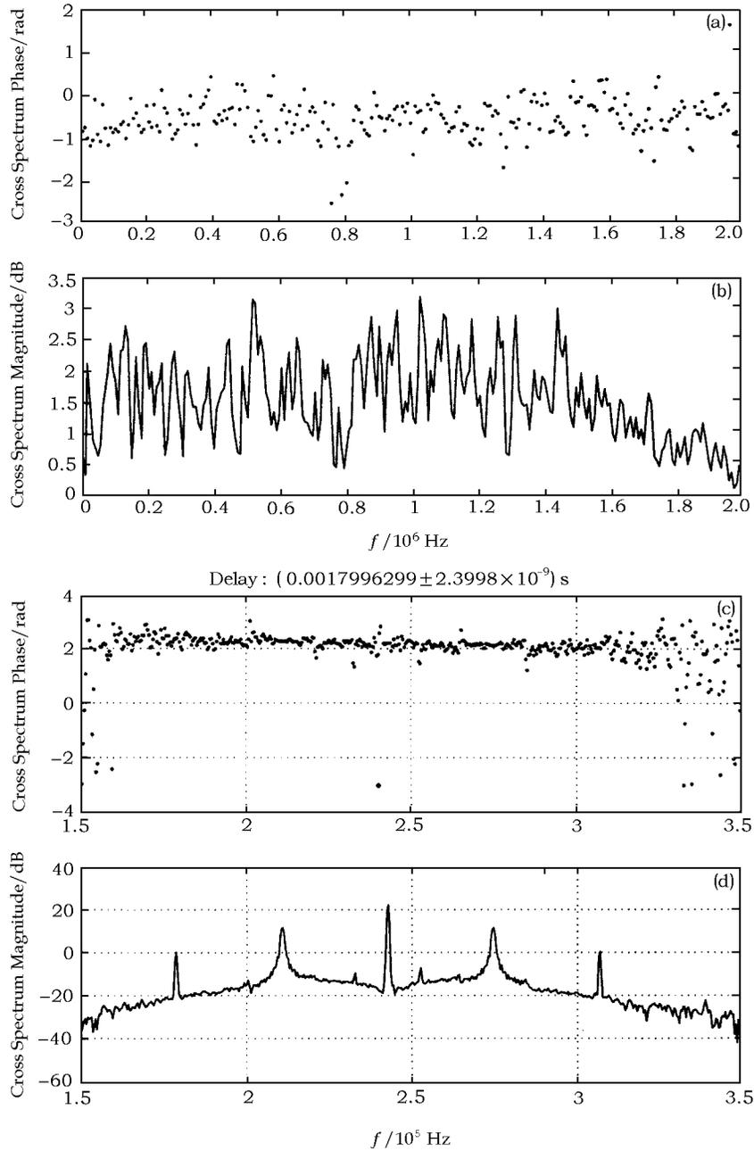
Fig. 4 Fringe checkout using software correlator, phase ((a), (c)) and amplitude ((b), (d)) spectra, DA193 ((a), (b)), GEO satellite telemetry signal ((c), (d))
