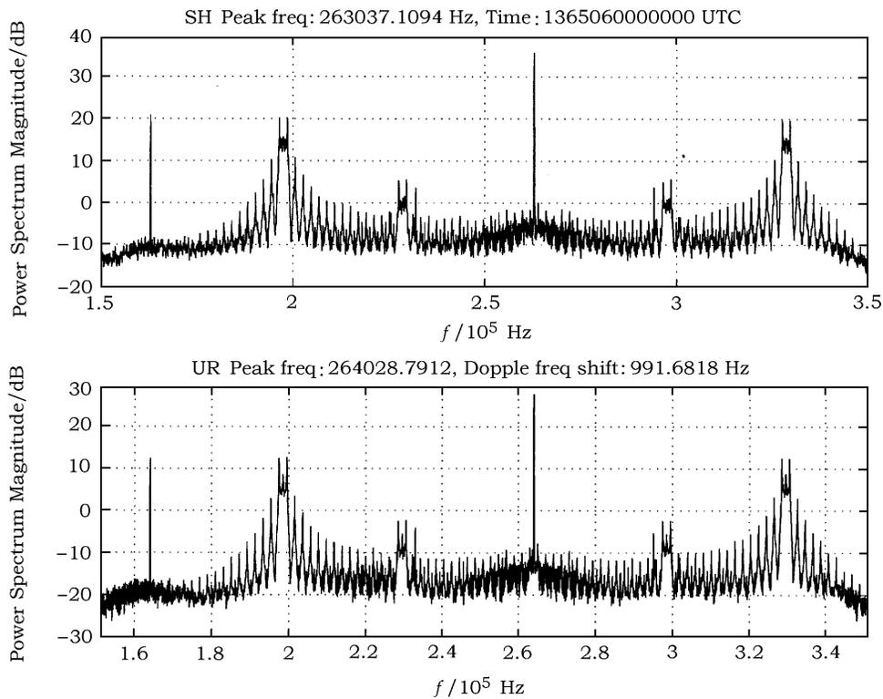
Fig. 5 Spectra of satellite downlink telemetry signals, Sheshan (up), Nanshan (down)
