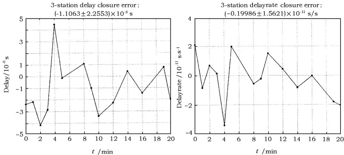
Fig. 12 3-station satellite observation delay closure error (left) and delay rate closure error (right)
