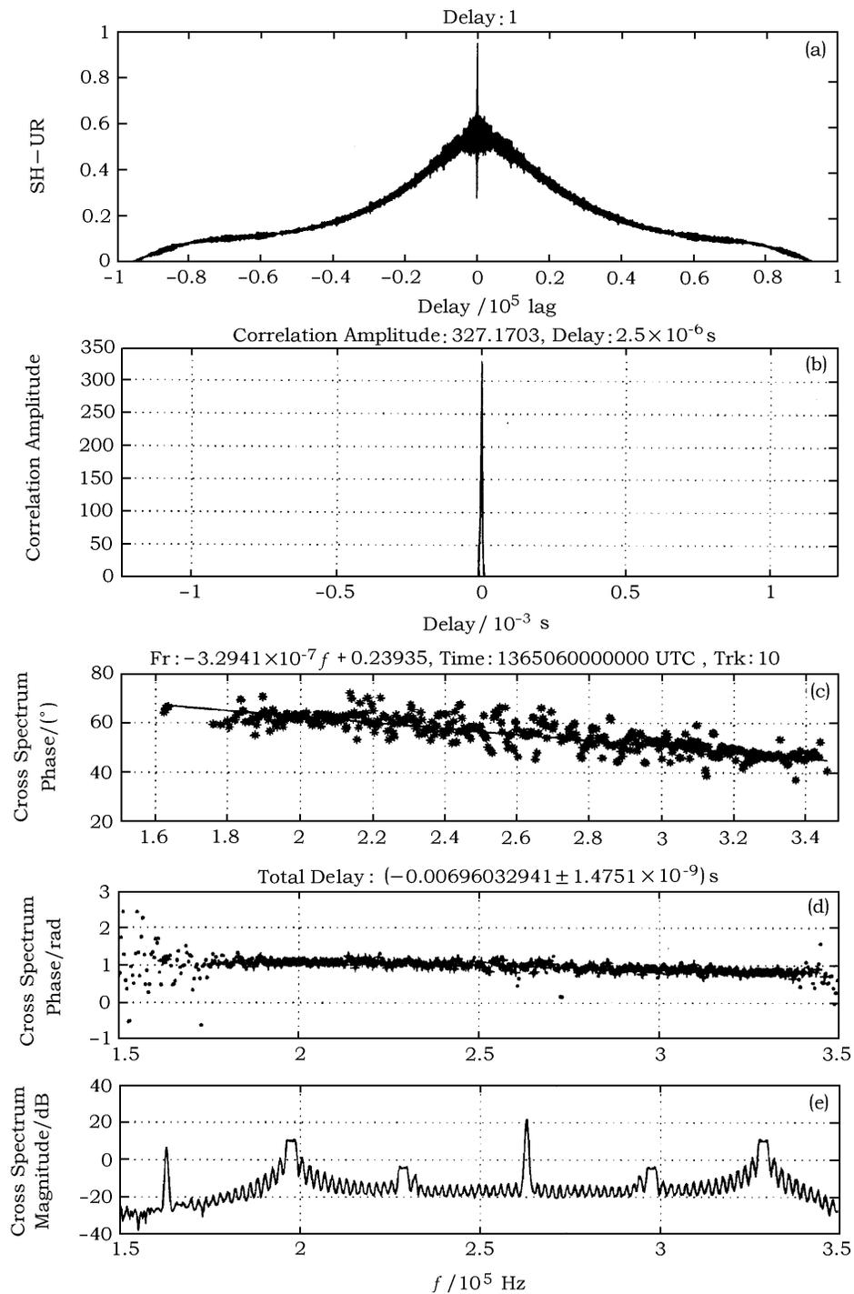
Fig. 7 Delay search window, XF method ((a), (b)), FX method ((c), (d), (e))
