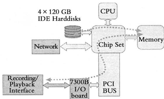
Fig. 1 Structure of CVN harddisk system
