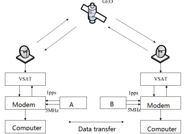
➢GPS Common View (CV) : Making satellite-differences between two stations, Satellite related error removed.
