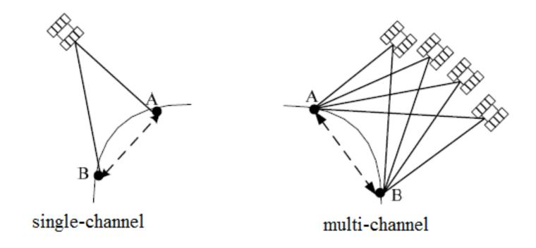
➢GPS All in View (AV) : Clock estimation using all satellites observed.
