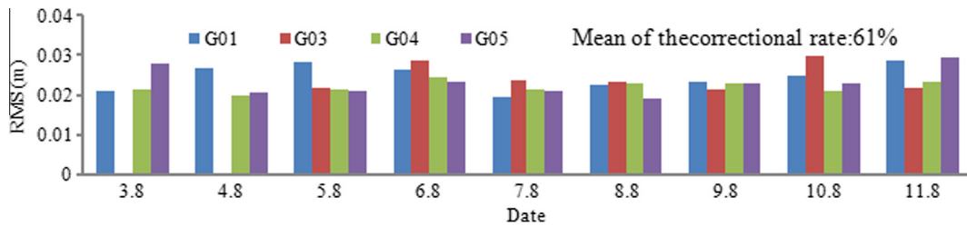
Fig. 12. RMSs of the predicted IFCBs compared with the estimated ones, for the time DOY 215-224, 2012. The axis is labeled DD.MM.
