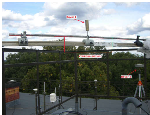
Fig. 2 The experiment field at GFZ, where Rover 1 (A17B) was set up on the horizontal linear table with scale panel to read the distances between the current and initial positions, and Rover 2 (A17D) was equipped with the device capable of adjusting the antenna height and recording the height changes
