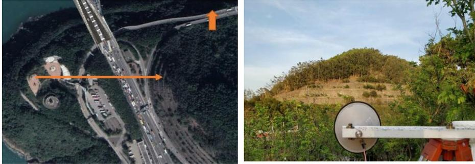
Slope monitoring with distance of 300m
