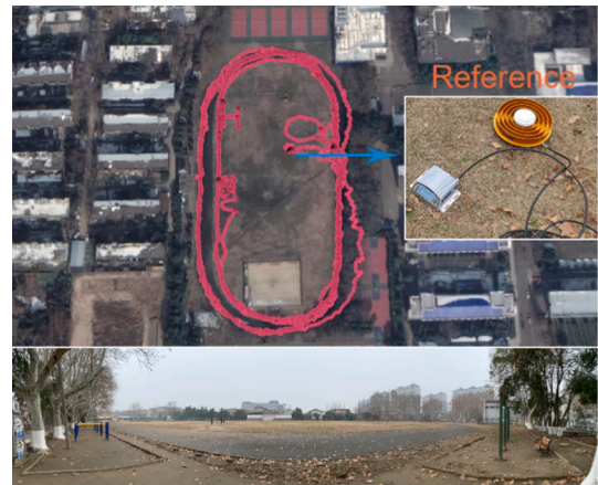
Fig. 10. Trajectory of the rover station and the location of the reference station.
