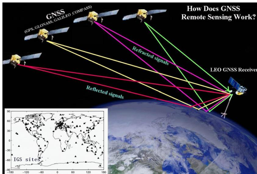
Fig. 3. Remote sensing using future denser GNSS network and more satellite constellations. The left lower corner shows the global IGS sites distribution.
