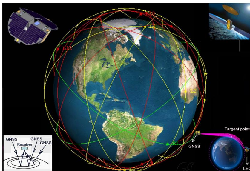
Fig. 4. CICERO (Climate Community Initiative for Continuing Earth Radio Occultation) with about 100 satellites (Yunck et al., 2007). The left lower corner shows the GNSS-Reflectometry and the right lower corner represents GNSS Radio Occultation.
