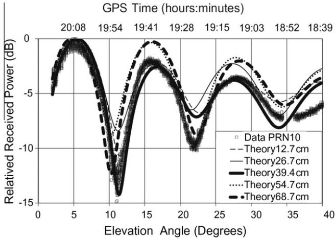
Fig. 2. Theoretical (lines) and measured (squares) elevation plots for a reservoir covered by a 0.3 cm thick snow layer on top of 12.7-, 26.7-, 39.4-, 54.7-, and 68.7 cm-thick ice layers with  $h = 50.5$  cm for the GPS satellite PRN 10 (Jacobson, 2010).
