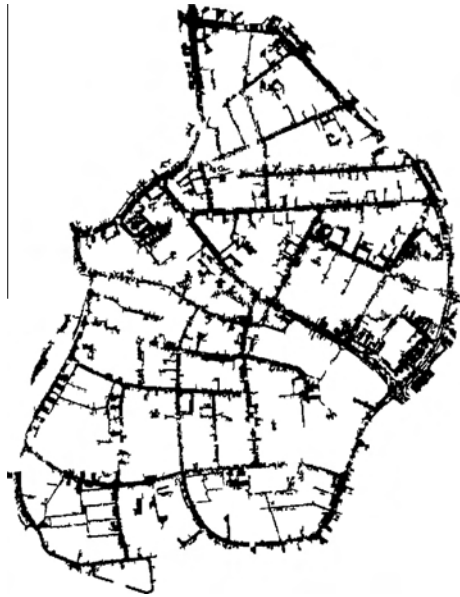
Fig. 4. Initial road rastered image. The road point cloud was first projected onto the XY plane and rastered into a binary image. Then a morphological closing operation was carried out to fill some holes. Finally, four connected analysis was applied to eliminate some non-road areas.
