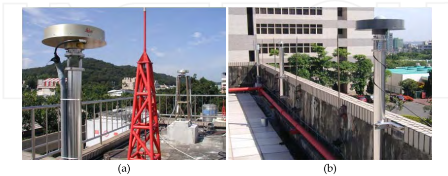
Figure 2. (a) Appearance of fixed stations; (b) Appearance of pillars of calibration base points [1]
