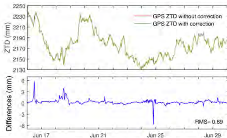
Figure 2. Time series of ZTD values ( top ) and differences ( bottom ) at the DIYB GPS station on days 168–180 in 2011.
