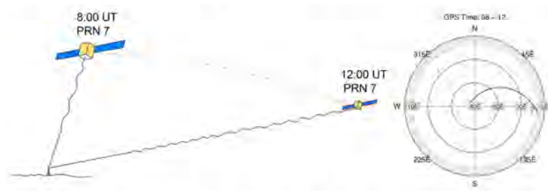
Figure 9. PRN 7 satellite visibility on day 167 in 2011 at ANRK station.
