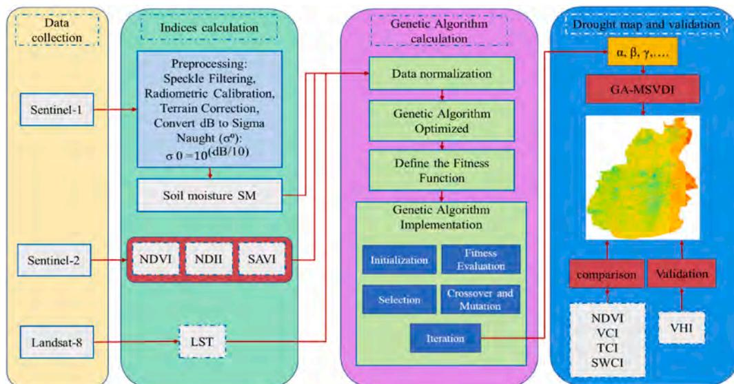
**Fig. 2.** A detailed flowchart illustrating the step-by-step methodology used to develop the Genetic Algorithm-Optimized Multispectral Soil-Vegetation Drought Index (GA-MSVDI). The process includes data acquisition, preprocessing, feature selection, Genetic Algorithm (GA) optimization, drought index computation, and validation against established drought indices.
